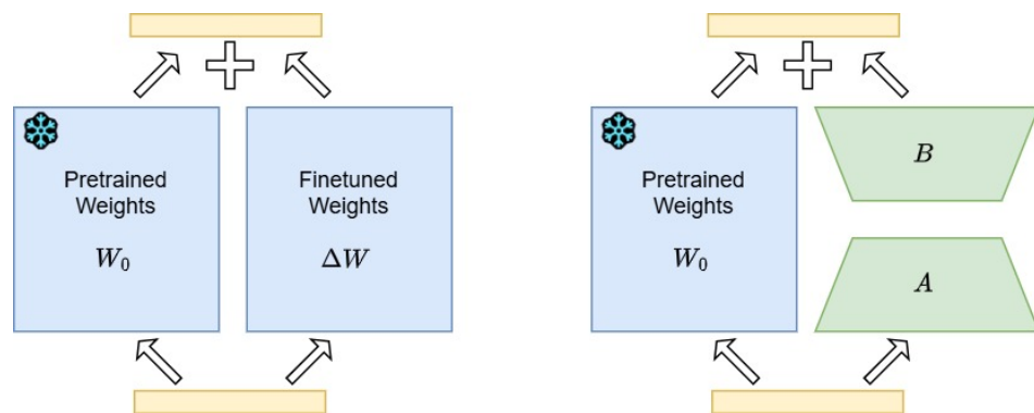
Figure 2. Illustration of the low-rank adaptation module.
