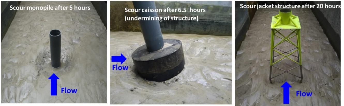
Figure 6. Scour near the pile’s foundation structures.
