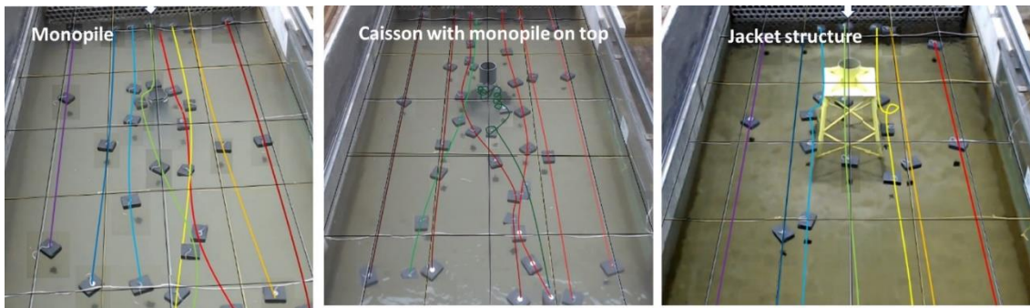
Figure 4. Flow lines for the 3 main experiments, obtained from tracking the position of near-surface floats (flow from top to bottom).
