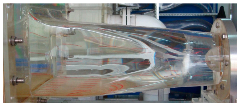
Figure 9. Photo of flow state of inlet passage.
