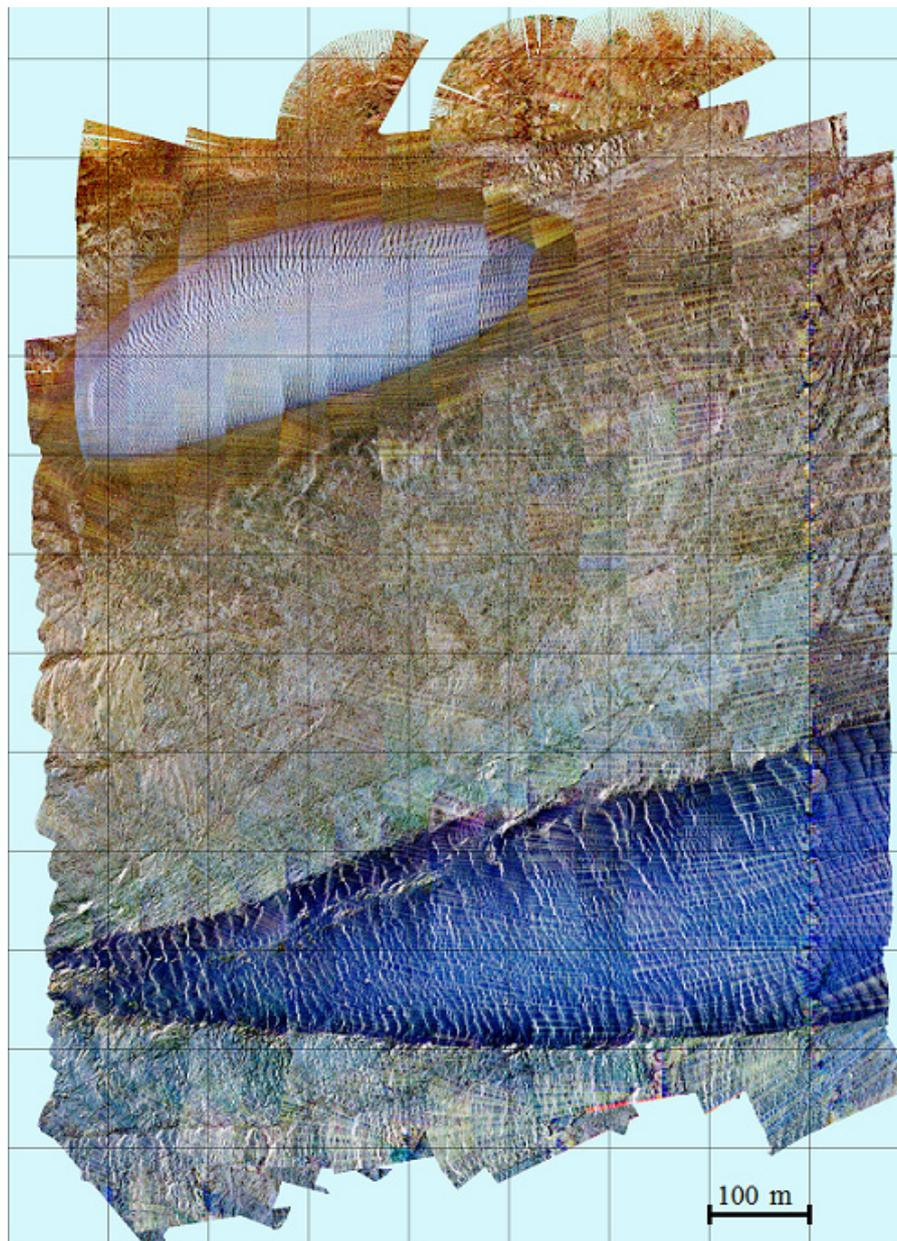
**Figure 7.** Swath montage chart of the seabed in the Inner Sound of the Pentland Firth. Fifteen swaths running north-south are overlain from west to east. The direction of ensonification is therefore principally to the west (left). Colour is encoded using the negative BGR method.
