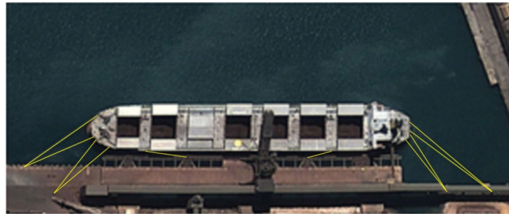
Figure 2. Panamax bulk carrier moored at Berth 5 with a typical mooring layout (mooring lines highlighted in yellow; spring lines and outer bow/stern lines are double; source: Google Earth).
