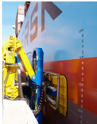
Figure 4. MoorMaster unit connected to a container ship (Source: Cavotec [12]).
