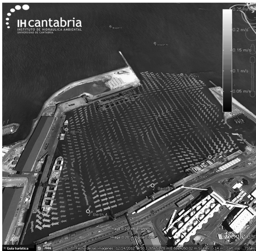
Figure 10. Snapshot for the maximum long wave-induced current of the 27 August 2007 inoperability event at Geraldton Harbor, obtained with the MANOLO model.
