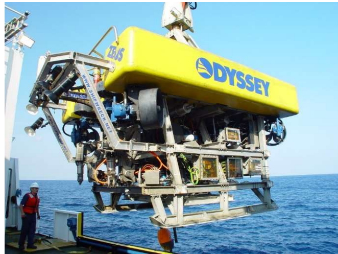
Figure 4. Odyssey's eight ton remotely-operated vehicle, called ZEUS.
