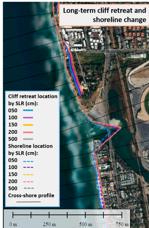
Figure 13. Long-term projected cliff retreat (solid colored lines) and sandy beach shoreline change (dashed lines) for various SLR at seaward lagoon entrance of Del Mar, California. In this projected management scenario, sandy beach erosion is limited to the urban boundary, and cliff retreat limited in locations with existing coastal armoring. Cross-shore transect/profile locations, at which long-term changes were derived, are shown by black lines. Cliff retreat projections are made only for transects with existing coastal cliffs/bluffs. Note that sandy beach projections converge for SLR 150–500 cm for a large portion of this area; all projections converge/show no change in locations where beach width is minimal (e.g., at the foot of the cliffs north of the lagoon mouth).
