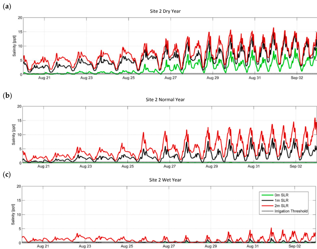
Figure 15. Surface salinity at site 2 in August with 0–2 m SLR: (a) dry year; (b) normal year; (c) wet year.
