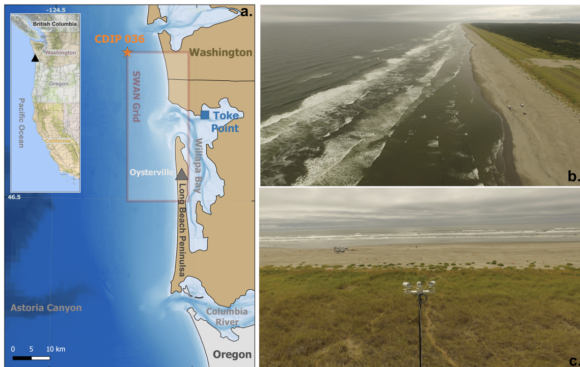
Figure 3. (a) Map of the Oysterville field site on the Long Beach Peninsula, WA, USA. The locations of nearby wave (Coastal Data Information Program (CDIP) 036), tide (Toke Point, WA), and wind measurements (Toke Point, WA) and the Simulating Waves Nearshore (SWAN) wave model domain used to transform offshore waves locally to Oysterville are also shown. (b,c) Aerial photos of nearshore, beach, and dune at Oysterville, WA taken on 9 August 2016 during low energy wave conditions ( H_s \sim 1.5 m). Photo (c) is taken from directly above the foredune crest where a camera mast system (shown) and meteorological station (not shown) were located during SEDEX 2 .
