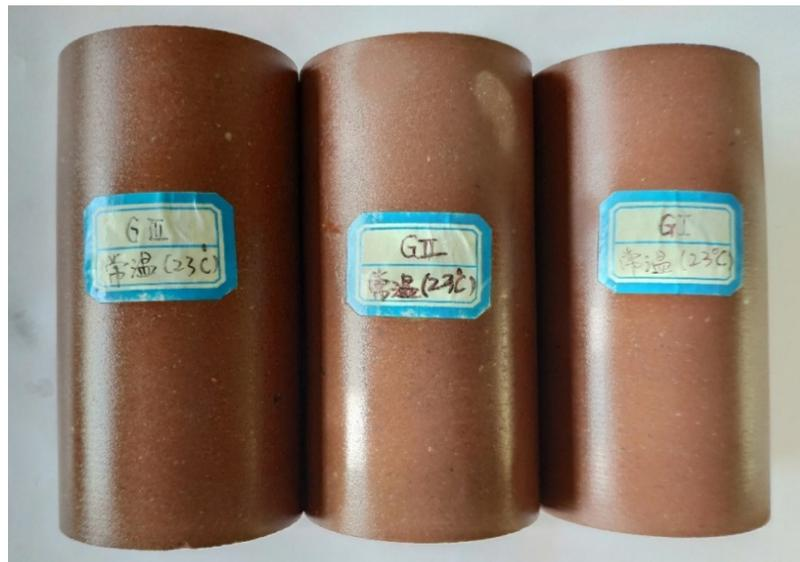
(b) Normal-temperature test specimens.
