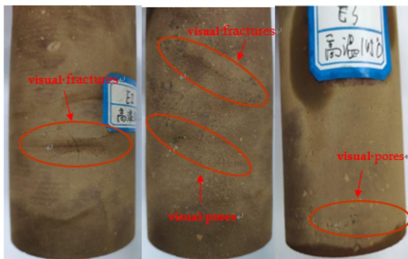
(a) High-temperature test specimens.
