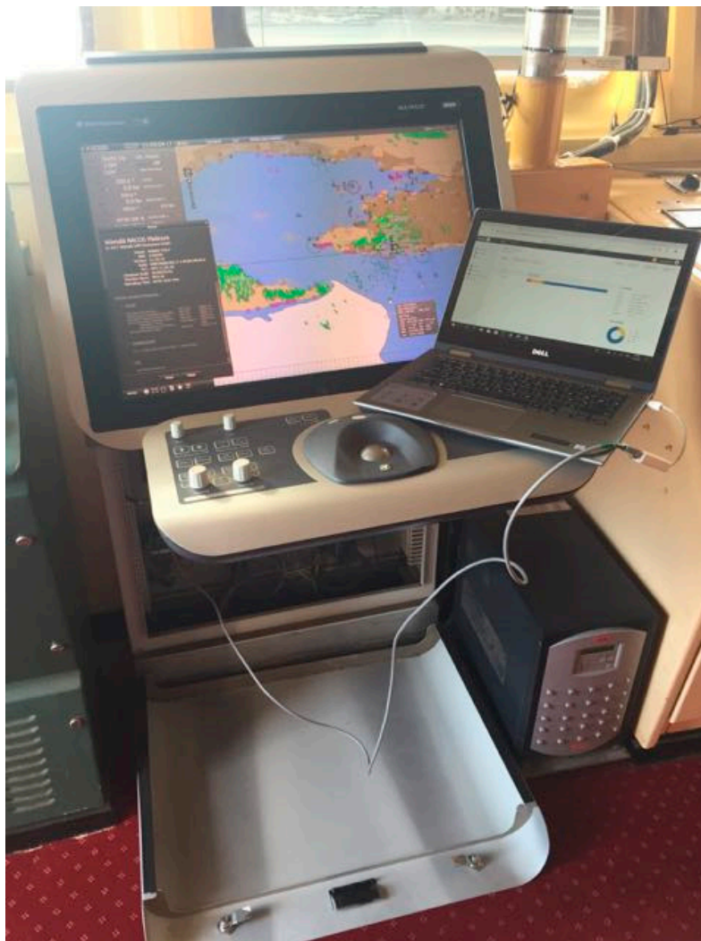
Figure 3. Testing setup for the INS cyber-vulnerability scanning.
