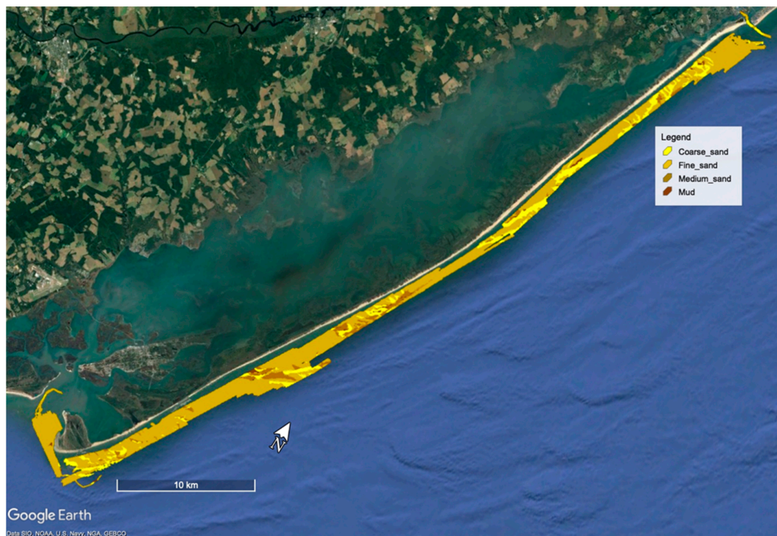
Figure 9. Sediment classification from 2014–2015 for the entire study area. Four sediment classes (coarse and medium sand, mud, and fine sand) were recognized and shaded with different colors. Mapping survey conducted 2014–2015.
