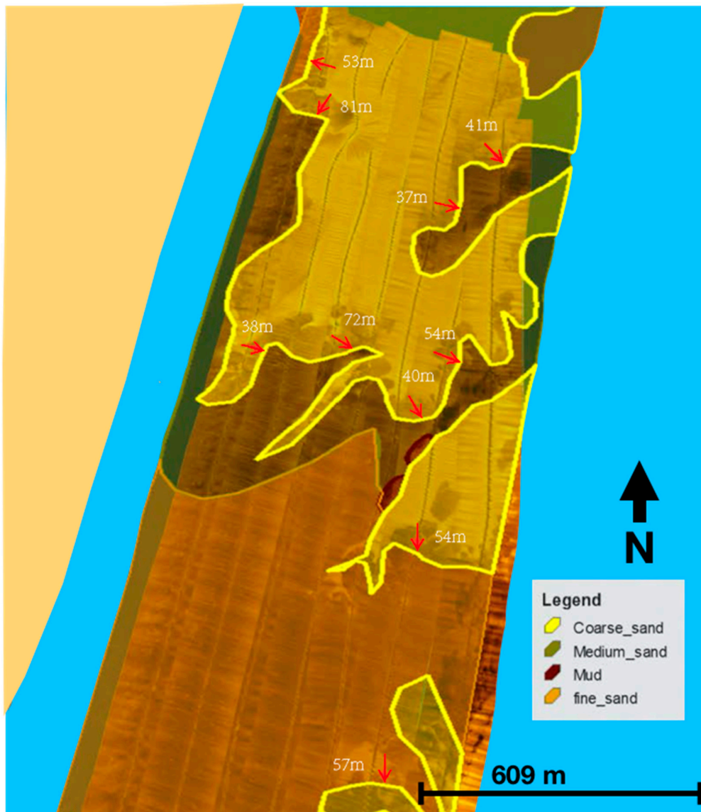
Figure 19. Temporal changes in sediment class boundaries, Assateague Island National Seashore, Maryland. The profile in the bottom is the side-scan sonar mosaics collected during May 2015. Shaded polygons on the top represent sediment classes inferred from the side-scan sonar mosaics collected during October 2015. Please note the west-south-eastward shift (38–57 m) in the boundaries of fine–coarse sand sediment classes.
