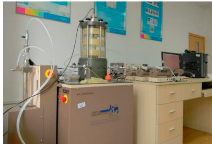
Figure 3. Dynamic triaxial test machine.
