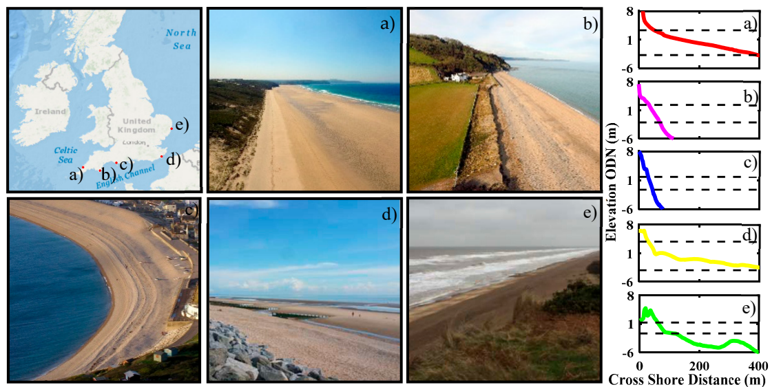
Figure 2. Location (top left corner), photographs (left), and representative profiles (to the right of the photographs) of (a) Perranporth (PPT), (b) Beesands (BEE), (c) Chesil (CSL), (d) Camber (CAM), and (e) Minsmere (MMR). Dashed black lines on the profiles represent mean high and low water spring tidal elevation. The Chesil photograph (c) is licensed under the Creative Commons Attribution-Share Alike 3.0 Unported license ( https://creativecommons.org/licenses/by-sa/3.0/deed.en ).
