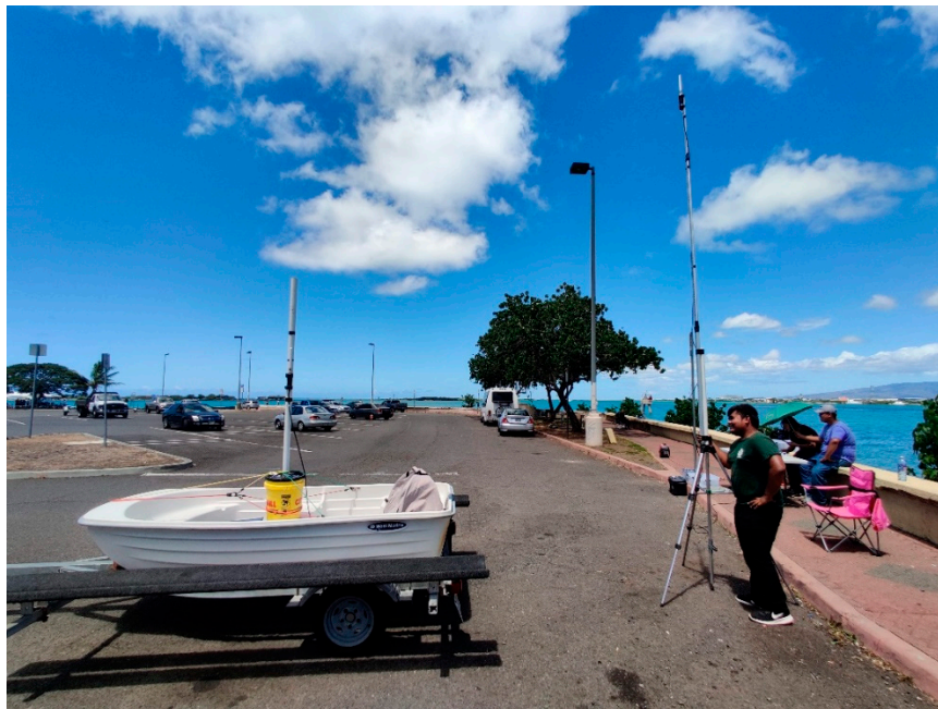
Figure 2. Over-land experimental setup. Ground station transmitting antenna (mounted on tripod, right), and trailered rigid tender serving as mobile station with receiving antenna (left).
