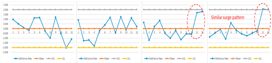
Figure 9. The control chart for deficiency 02 (2015–2018).
