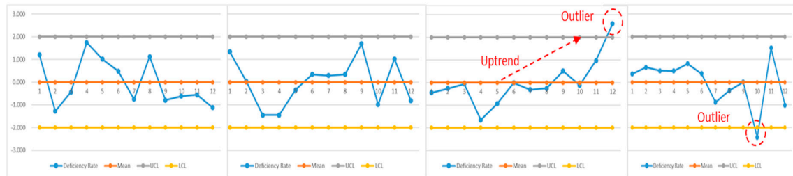
Figure 13. The control chart for deficiency 10 (2015–2018).
