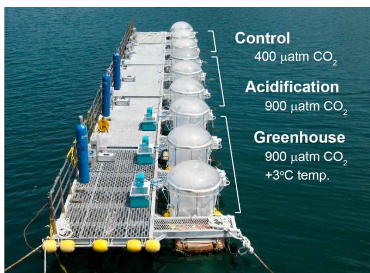
Figure 1. Photograph of the floating raft, \text{pCO}_2 concentration regulation units, temperature regulation units, and enclosures of the mesocosm facility. Design and performance of the facility have been described in detail elsewhere [26,27].
