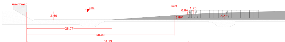
Figure 6. Sketch of the experimental layout. The 2-D numerical model mimics this layout to a great extent. Conversely, the 3-D model has an open boundary for wave generation at the inlet, i.e., at x = 50 m.
