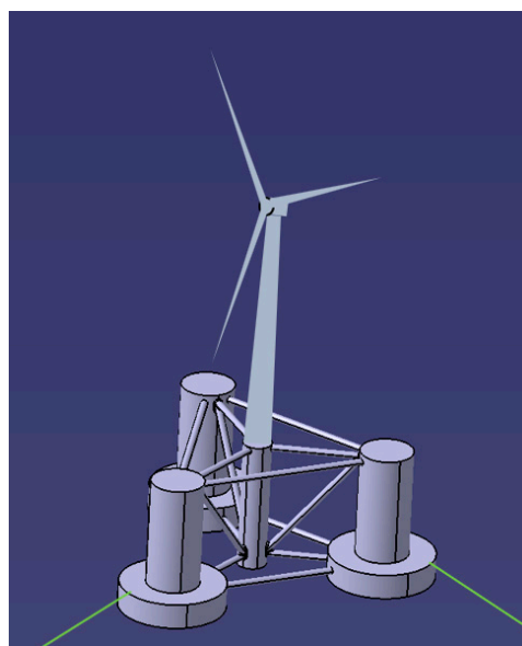
Figure 1. OC4 semi-submersible floating offshore wind turbine (FOWT) system.
