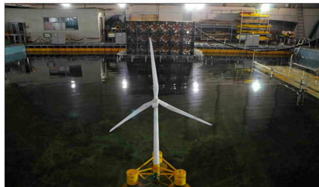
Figure 2. Model tests of the 5 MW semi-submersible platform model in the water tank of Ulsan University (UOU).
