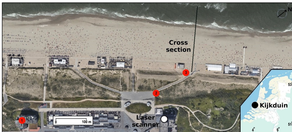
Figure 2. Overview of the Kijkduin study area with the laser scanner and cross-section used in the analysis. Red points (numbered 1–3) indicate the reference object locations used for georeferencing (see Section 2.2).
