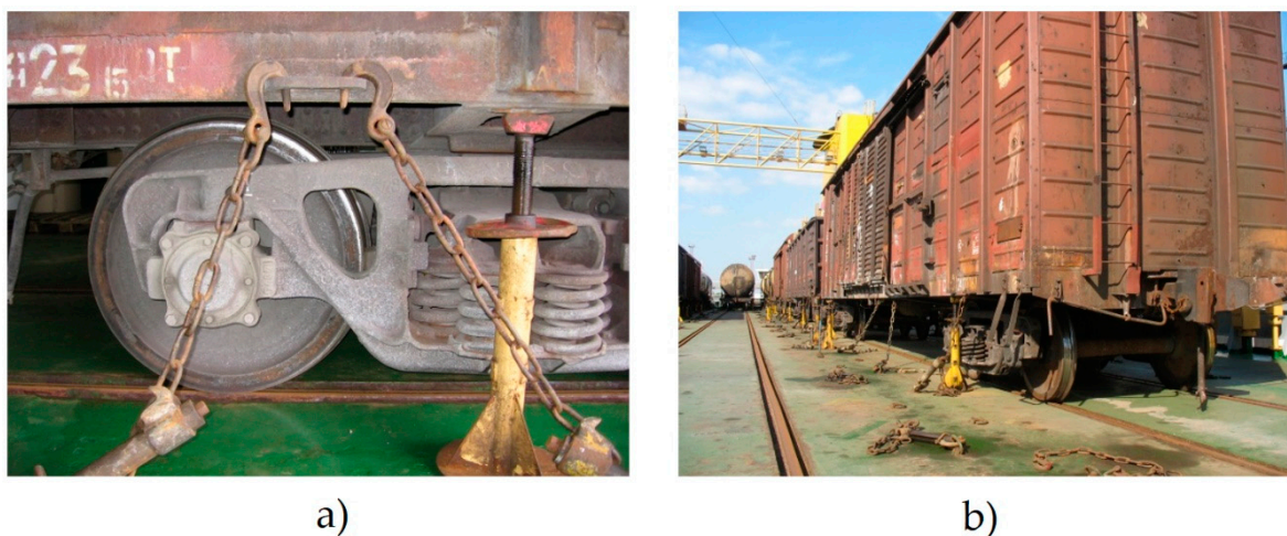
Figure 2. Securing wagons on a rail ferry (a) open wagon; (b) covered goods wagon.
