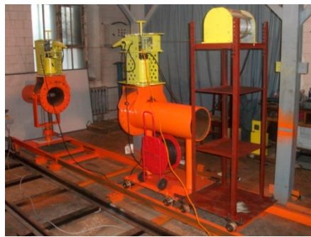
Figure 1. Measuring device based on the outer circle positioning of the pipeline.
