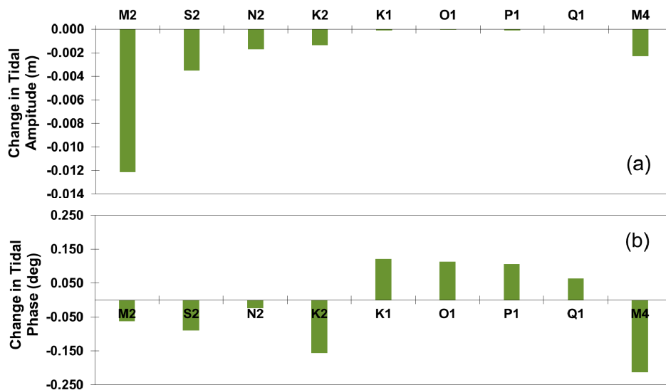
Figure 14. The changes in tidal amplitude (a) and phase (b) at the NOAA tidal gage near Anchorage, Alaska, as a result of power extraction in S2.
