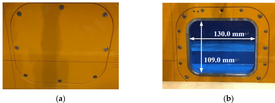
Figure 2. Damage opening: (a) intact state with a lid; (b) damage state without a lid.
