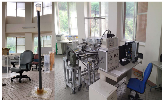
Figure 6. The simple experimental set up of OWT with a tuned liquid damper (TLD) on top.
