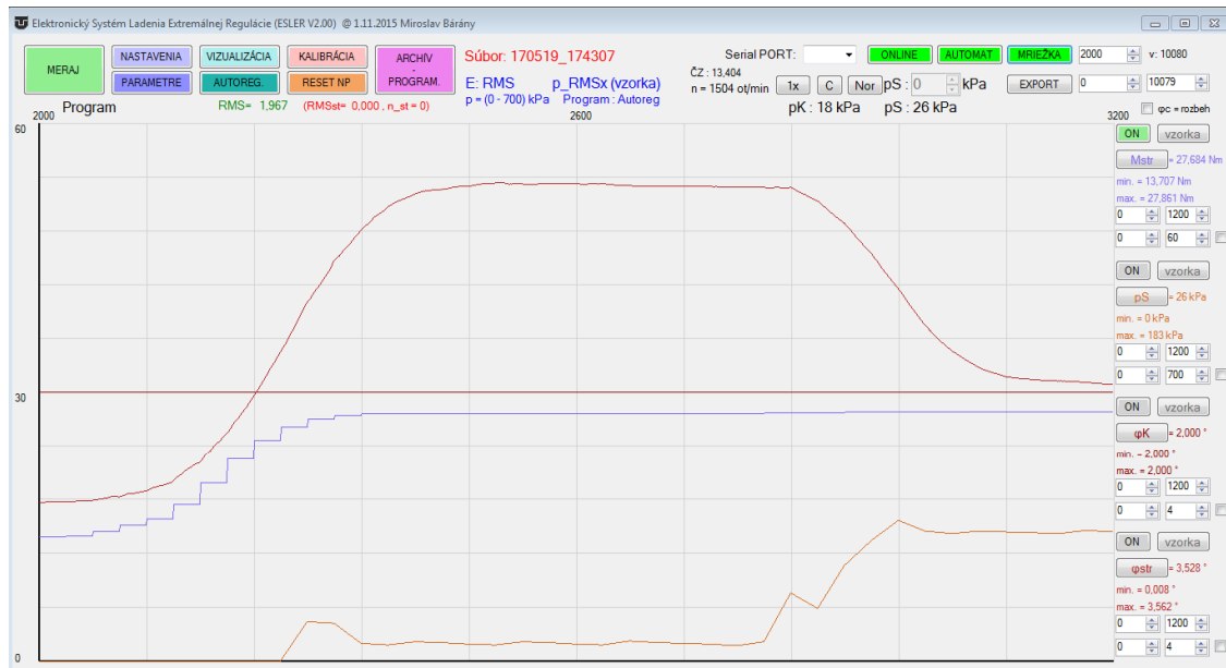
Figure 11. The graphical user interface of the electronic constant twist angle control system.
