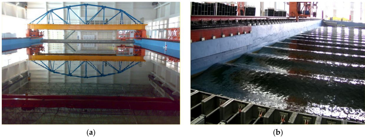
Figure 13. Towing tank and its wave-making equipment. (a) Towing tank at Harbin Engineering University. (b) Wave-making equipment in towing tank.
