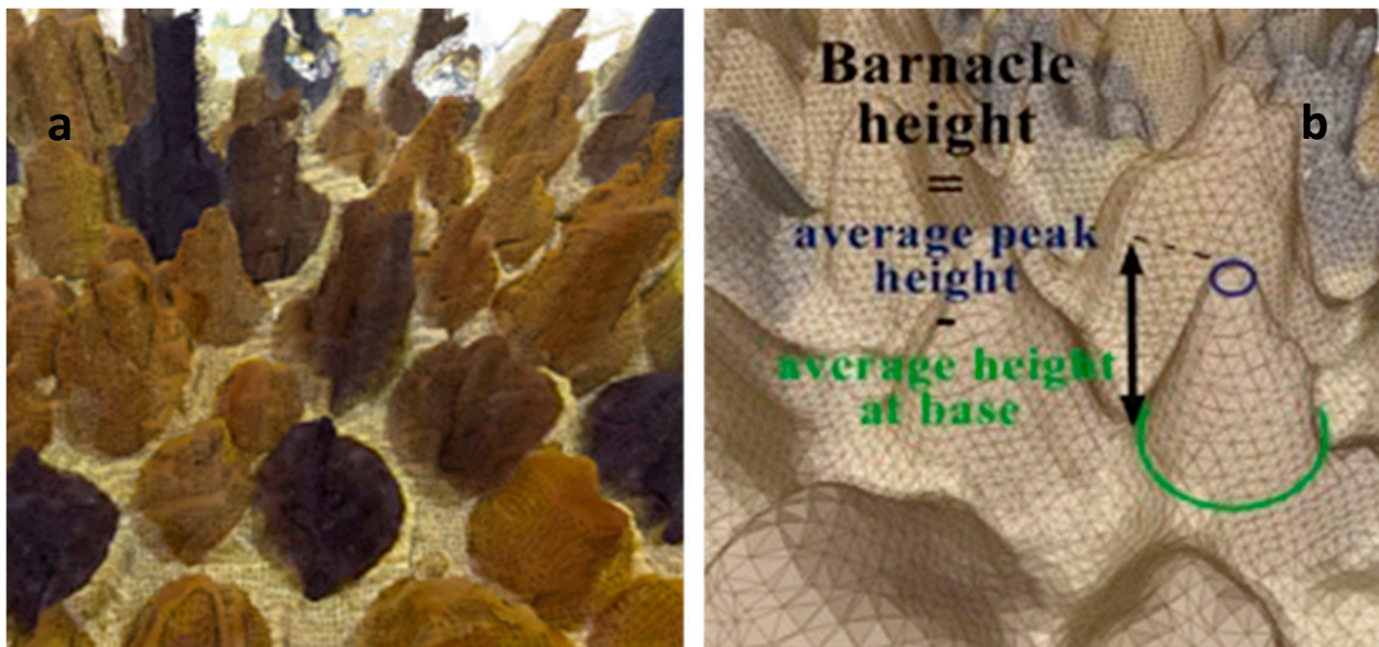
Figure 13. Numerical mapping (a) and computation of specimen height (b).
