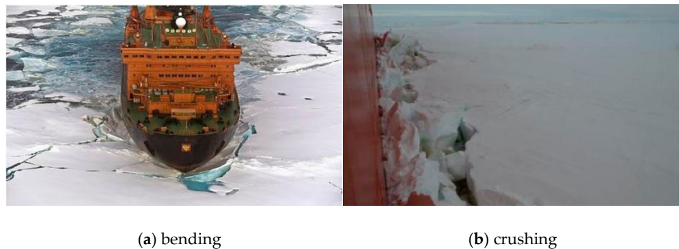
Figure 11. Breaking mode of level ice ( www.eworldship.com , accessed on 19 July 2014).
