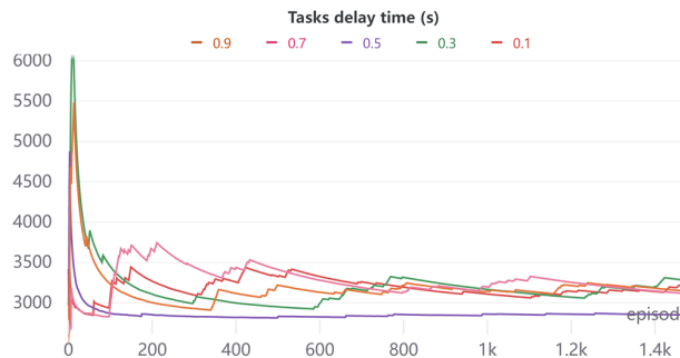
Figure 7. Task delay time of CDA algorithm with different values of \beta .
