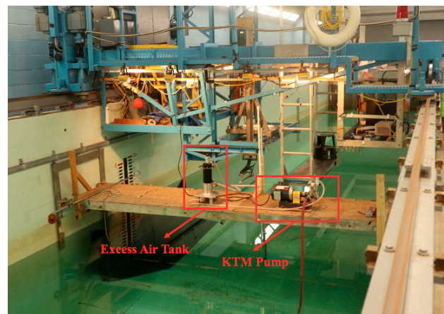
Figure 5. The setup of the Nikuni KTM pump in the tow tank.
