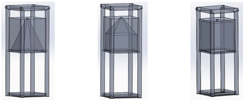
Figure 4. Consideration for various shapes of air-chamber of the OWC wave energy converter installed in an offshore template structure.
