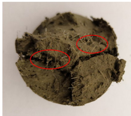
Figure 9. Sectional view of PCC after failure.
