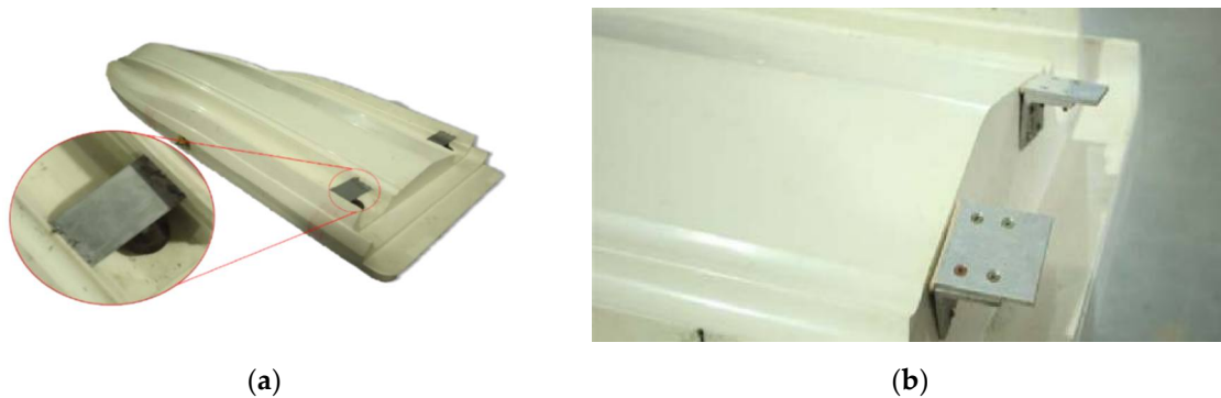
Figure 4. The installed hydroflap and stern flap at the hull tail. (a) Hydroflap; (b) stern flap.
