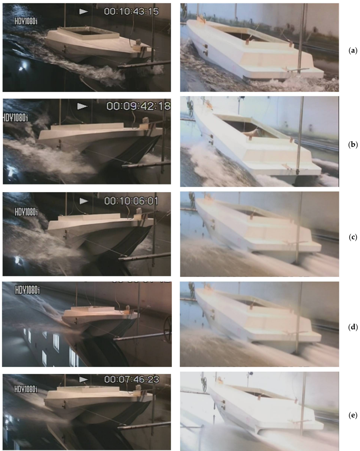
Figure 6. The screenshot of the towing test of C-B90-85 at different velocities. (a) Fn = 0.95 ; (b) Fn = 1.91 ; (c) Fn = 2.38 ; (d) Fn = 4.77 ; (e) Fn = 7.15 .
