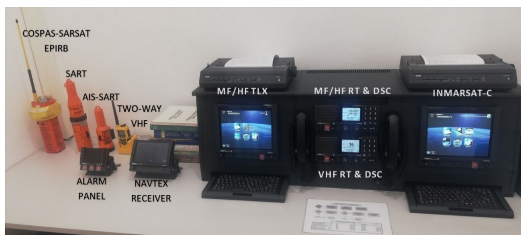
Figure 1. Typical Global Maritime Distress and Safety System (GMDSS) radio station and equipment for sea area A3.
