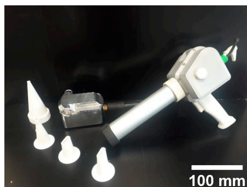
Figure 7. Underwater mortar injection tool (Tech4Sea srl 2020).
