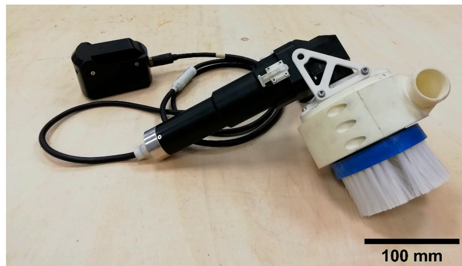
Figure 5. The cleaning tool with the suction brush accessory (Tech4Sea srl 2020).
