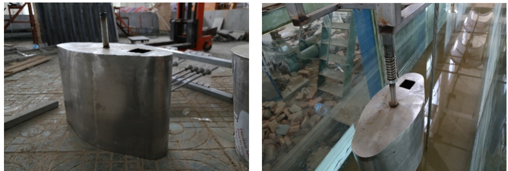
Figure 3. The elliptical cylinder of oscillating buoy.
