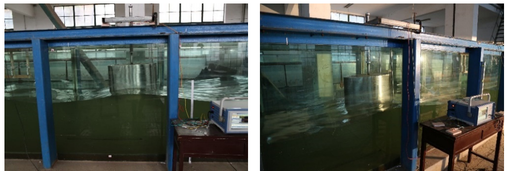
Figure 5. Installation of WEC experimental device in flume.
