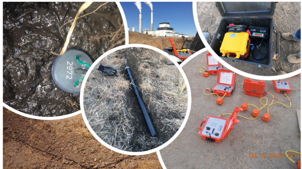
Figure 8. Pictures of the various electromagnetic sensors and acquisition systems in field settings. At the top left is an electrode used for the electric field measurements. At the top center is the acquisition system near a power plant followed on the top right followed by a closer view of the system, web access box, and battery in a field container. Below on the bottom right are several systems during a test with seismic 3-component geophones connected. In the center is a magnetic field sensor (induction coil) and in the bottom left a magnetic field sensor implemented by a large multi-turn air loop.
