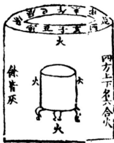
Figure 15. The cabinet of the fountain and the iron rack with three legs (Zhao 1988, p. 249c).
