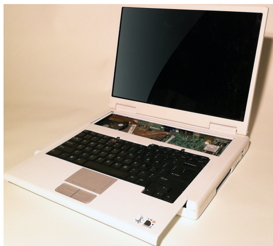
Figure 5. Dismantle laptop by Isaac Alves and Joseph Lapke can be fully disassembled in about ninety seconds. Photo by Lobos.
