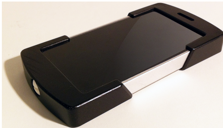
Figure 7. Design for Repair phone by Fahmi Dereinda, Patrick McKernan and Gregory Townsend allows for easy access to internal parts while providing additional protection if dropped. Photo by Lobos.
