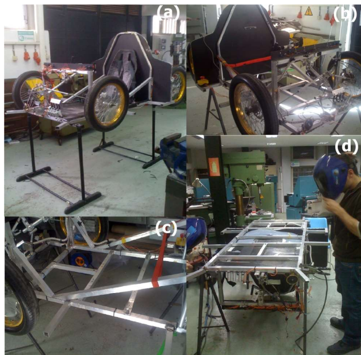
Figure 9. Electric car: (a) final product; (b,c) semi-finished product; and, (d) welding of the front and the rear semi-axle kits on the chassis; [3,7].
