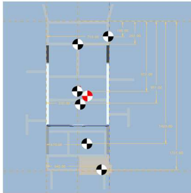
Figure 7. Top view of the electric car's centre of gravity.
