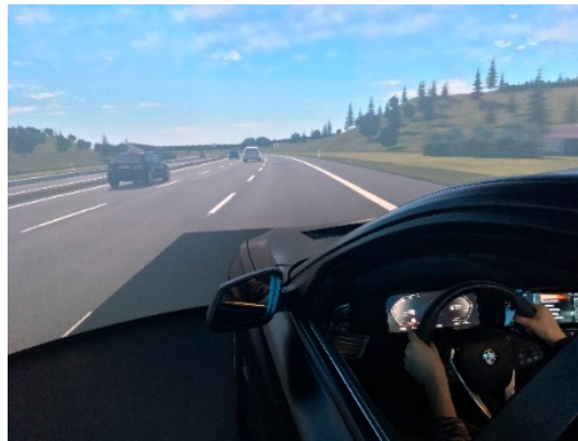
Figure 1. Static driving simulator mockup used in the present study.
