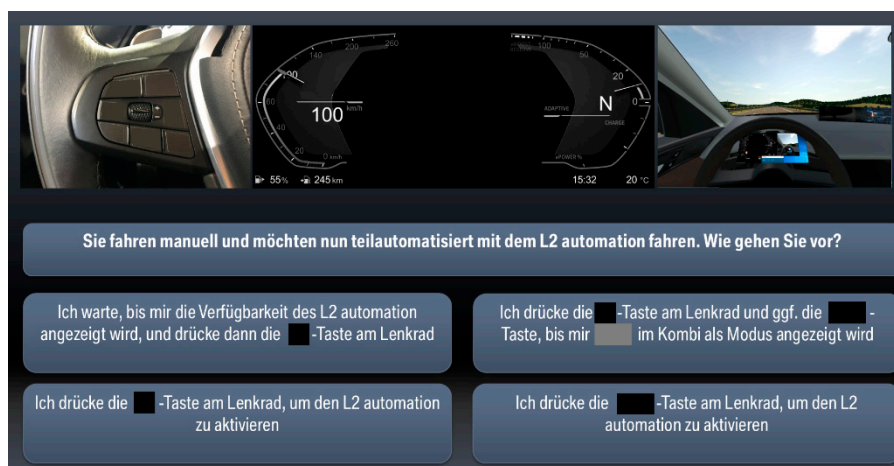
Figure 3. Layout of interactive tutorial with operating element (upper left), instrument cluster (upper middle), driver’s view (upper right), user task, and four alternative answers.
