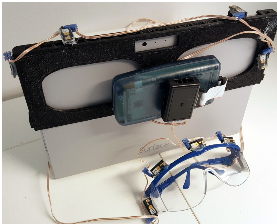
Figure 8. The apparatus: a tablet PC covered with a 3D printed frame. The frame is mounted with the LED illuminative markers and their unit driver with batteries. A pair of safety goggles equipped with LED markers is connected to the same driver unit.
