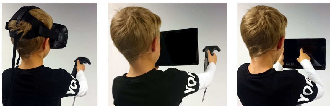
Figure 1. Three examples of Augmented Reality (AR) interaction: head mounted display and wand, hand-held and wand, and hand-held with touch.
