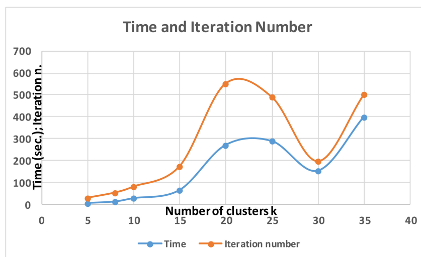
Figure A1. Time and iteration number versus the cluster number k (image processing of the same image).
