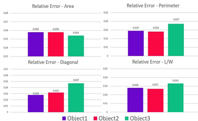
Figure 9. Absolute error for each of the measurements tested by the proposed heuristic calibration method.
