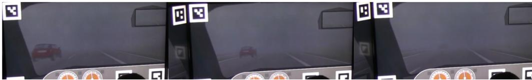
**Figure 5.** Visibility in the foggy scenarios. Vehicles disappear at a distance of approximately 33 m.
