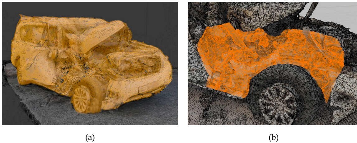
Figure 9. A generated 3D mesh objects of the vehicle 3D model in Blender (a) measuring the volume of the whole vehicle body (b) measuring the deformation volume of the collided frontal part of the vehicle.
