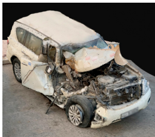
Figure 8. Photogrammetrically reconstructed 3D model of a real collided vehicle in Kuwait in the Alrabiya area.
