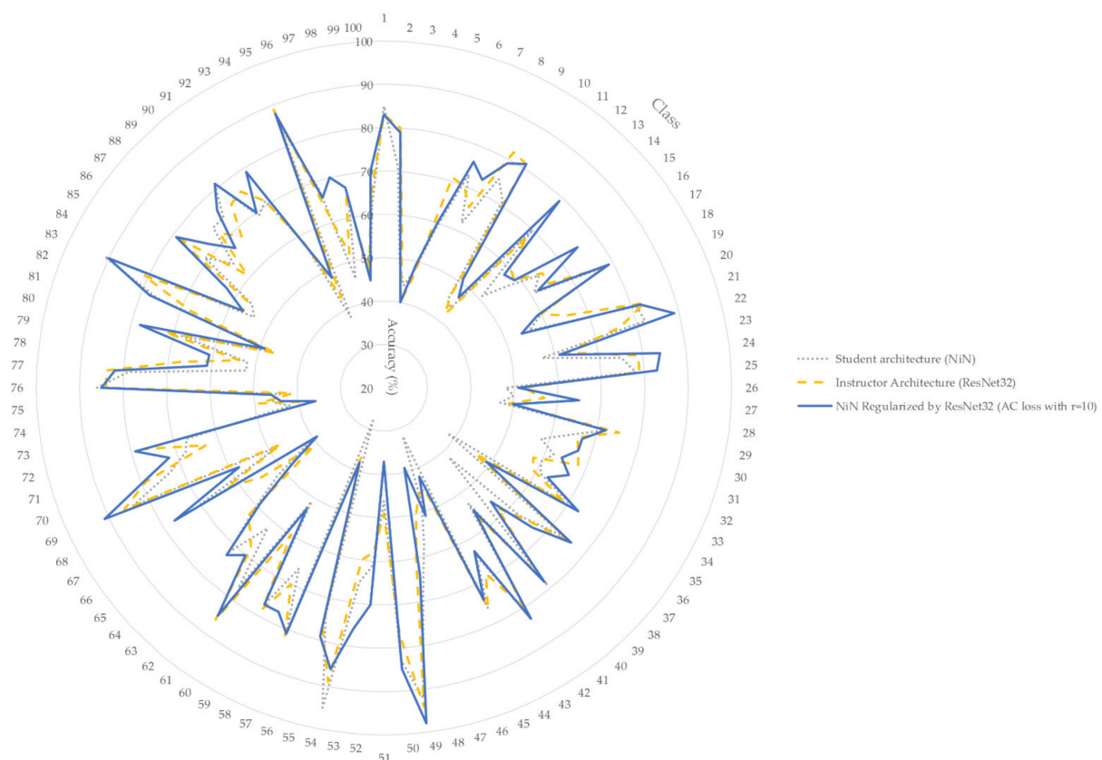
Figure 3. Class-wise accuracy obtained by reference NiN, ResNet32 and regularized NiN via AC loss in CIFAR100.
