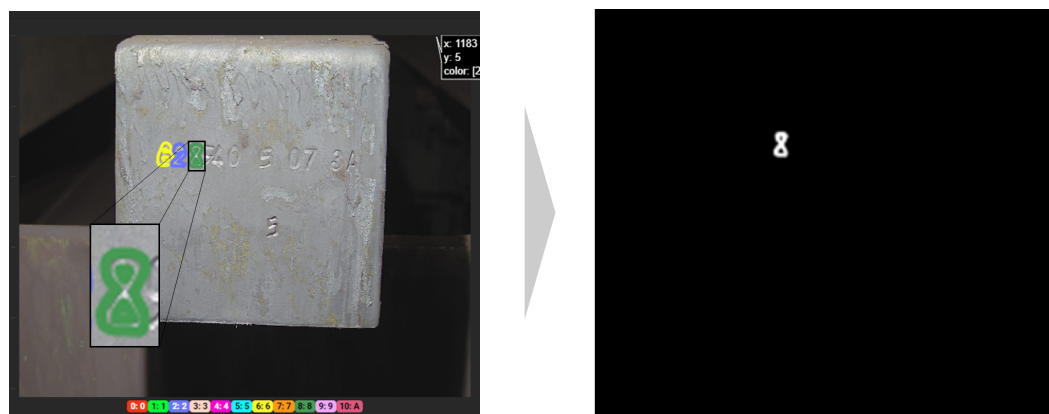
Figure 1. Conversion of a polygonal shape into segmentation mask (left: polygon of digit 8, right: mask of digit 8 as binary array).
